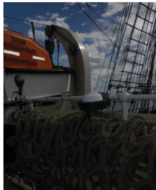
Figure 3. Position of the GPS antenna on the boatdeck
